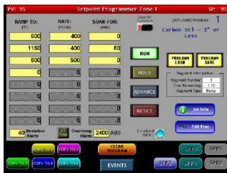
Setpoint Programmer Screen View in Advanced Mode on XTX
